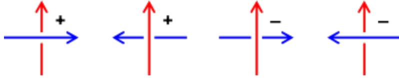
FIGURE 5. Signature of a crossing for the computation of the linking number.
